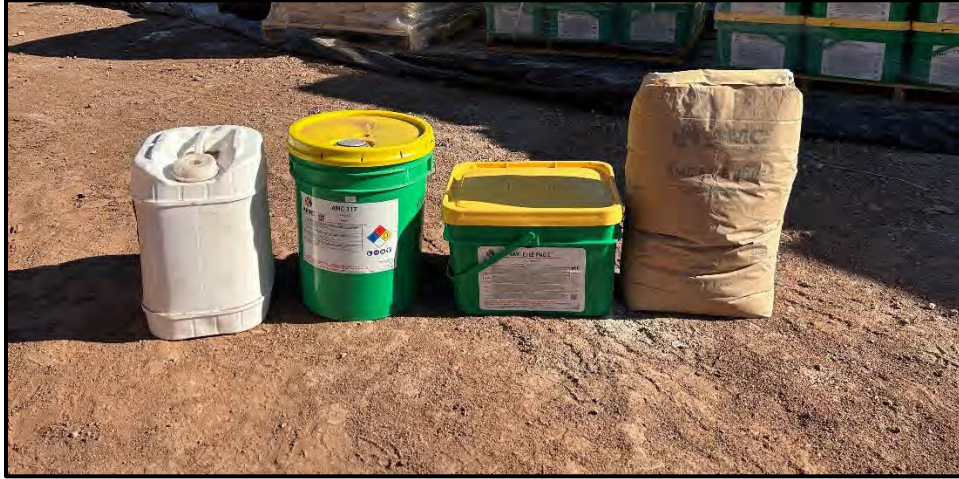
Figure 2-13. Typical containers and storage of drill mud additives on exploration drill pad.
