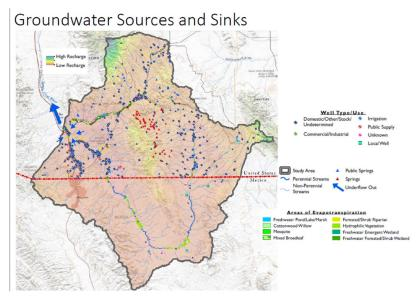
This slide [left] shows the location of the springs and wells. This data, together with those predicted dewatering and predicted pathways from the mine, is where you will identify the impacts of dewatering.
