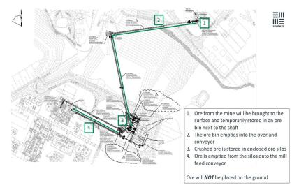
This picture [above] is an aerial plot plan of where the main shaft is on the property. This line traces the overland conveyor that takes ore to the processing plant. The ore will go directly from shafts to conveyor belts and then directly into the closed silos. We're not going to put the ore on the ground, at any point. It will be kept in the system to mitigate any dust exposure, keep things intact, easily processable, and relatively short residence time on the surface.
