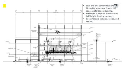
The filter cake drops straight into a half pipe container. Someone will take a product sample, to test for moisture and quality, moisture so that we ensure that it's safe for ship cargo holds. And then it is closed and sealed. Next is a truck and container wash. This is done within a covered building. All that water is blended into the sump pump on that concrete container and then goes back into the water recirculation that's used for processing.
